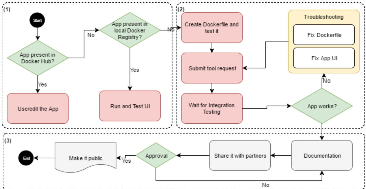
Figure 9: Running and Integration of a Docker Engine
